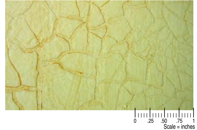
Step 1: Proceed® Low Absorbency Base Coat Step 2: 2 rolled coats Proceed® Cracking Size Step 3: Proceed® Transparent Cracking Glaze 100 sq. ft. (thinner application) coverage per gallon
