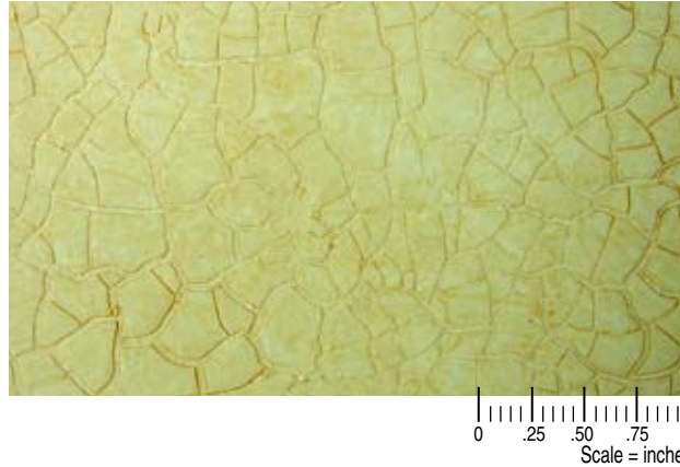
Step 1: Proceed® Low Absorbency Base Coat Step 2: 1 rolled coat Proceed® Cracking Size Step 3: Proceed® Transparent Cracking Glaze 100 sq. ft. (thinner application) coverage per gallon
